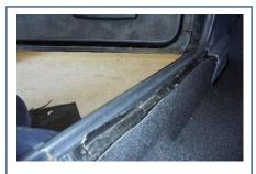
Trim the carpet down around the sill so it is in line with the top of the sill, and glue.
