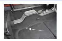
Then locate the seat belt holes in the tunnel, again make a hole in the carpet big enough to fit the bolt through. The seat belts can now be screwed into place.
