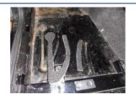
Use part's 3 – the floor filler felt to fill in the pressings pressed into the floor pan. These can be glued in place on their respected sides.
