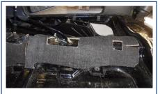
Secondly use number 2 – the rear tunnel section. Line up the cuts in the underfelt along with the tunnel and glue down.
