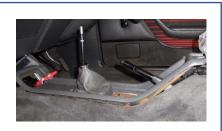
Unscrew the gear lever knob and lift off the console top, this will then allow you to lift out the console pocket.
