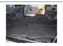
Starting with the passengers side first, lay this segment into the car.
