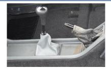
Screw the screws back in-in front of the gear lever and hand brake lever, place the blanking cap back on along with the facia in front of the hand brake lever, also refit the gear lever knob.
