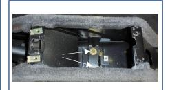
The console can now be put back into the car, start with refitting the console pocket and screw down.
