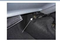
Feed the carpet in and under the heater matrix.
