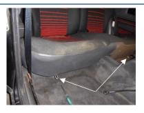
Remove the rear seat base by undoing the 2 screws either side.
