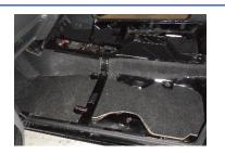
Pieces number 5 – the rear floor well sections, can be laid into place on the floor well and glued in. Minimal trimming if any is needed.
