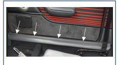
Next you will need to undo the four screws which hold on the sill plates, remove the sill plates from both sides of the car.
