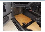
Now the carpet has been fully removed we can focus on removing the underfelt. Remove all of the pieces on the floor first.
