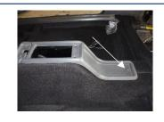
The rear section of the console can now go back in, however only fasten the back screw, the blanking plug can be refitted on top.
