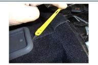
Next, locate the center of the transmission tunnel and cut both sides of carpet until they sit flush, then pull back and glue down to create a smooth finish.
