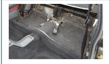
The rear seat base section can now be glued down into place.
